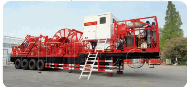
SLG380 trailer-mounted coiled tubing units
