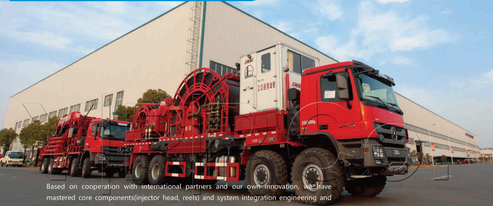
SLG380 coiled tubing units (main unit plus auxiliary unit)
